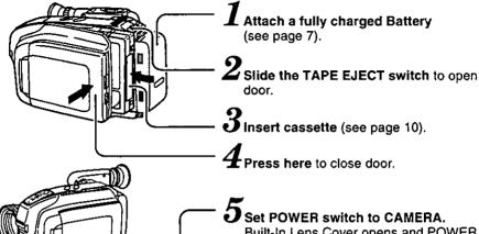
Set POWER switch to CAMERA. Built-In Lens Cover opens and POWER Lamp lights.
