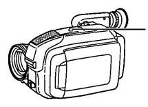
Press the BACKLIGHT button while recording.
