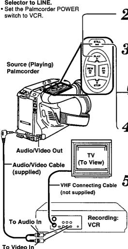
Insert a pre-recorded tape into the Palmcorder and a blank tape with a recording tab into your VCR
