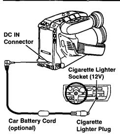
Connect a PV-C16 Car Battery Cord (optional) to DC IN on the Palmcorder.
