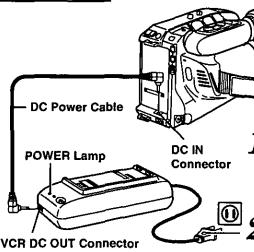
Connect VCR DC OUT on the AC Adaptor to DC IN on the Palmcorder with the DC Power Cable (supplied).
