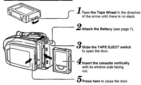
• To remove the cassette, slide the TAPE EJECT switch.
