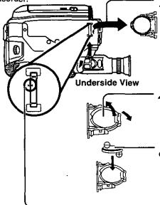
While pinching the stopper tabs, pull the Battery Tray out of the Battery Compartment.
