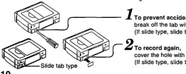
To prevent accidental erasure. break off the tab with a screwdriver. (If slide type, slide tab open.)
